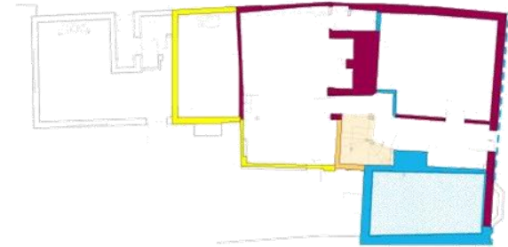
c.1787 Comprehensive period of modernisation, most likely in response to the fire protection measures put in place after the fires of the early 18C. The southern end is rebuilt in brick, a chimney added, and the front elevation is clad in mathematical tile. The entry is moved to the front of the house
