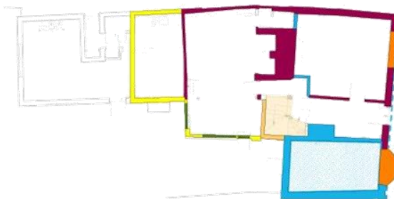
c.1920 - 1930 Adaptation of western reception room including modification/addition of windows and doors to south. propping of large beam and ledged and braced doors added
