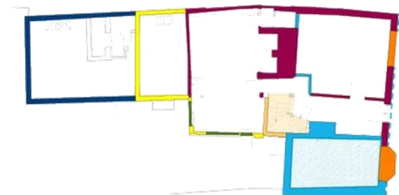
c.1960-1970 Addition of 2 storey extension to west housing kitchen and master bedroom
