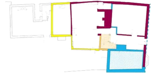
c.1787 Comprehensive period of modernisation, most likely in response to the fire protection measures put in place after the fires of the early 18C. The southern end is rebuilt in brick, a chimney added, and the front elevation is clad in mathematical tile. The entry is moved to the front of the house
